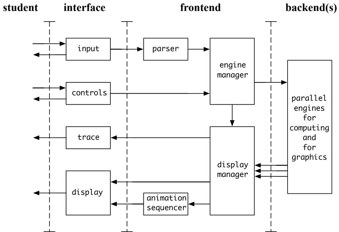
**Figure 24: Block Architecture for the Boundary Animation Tool**
