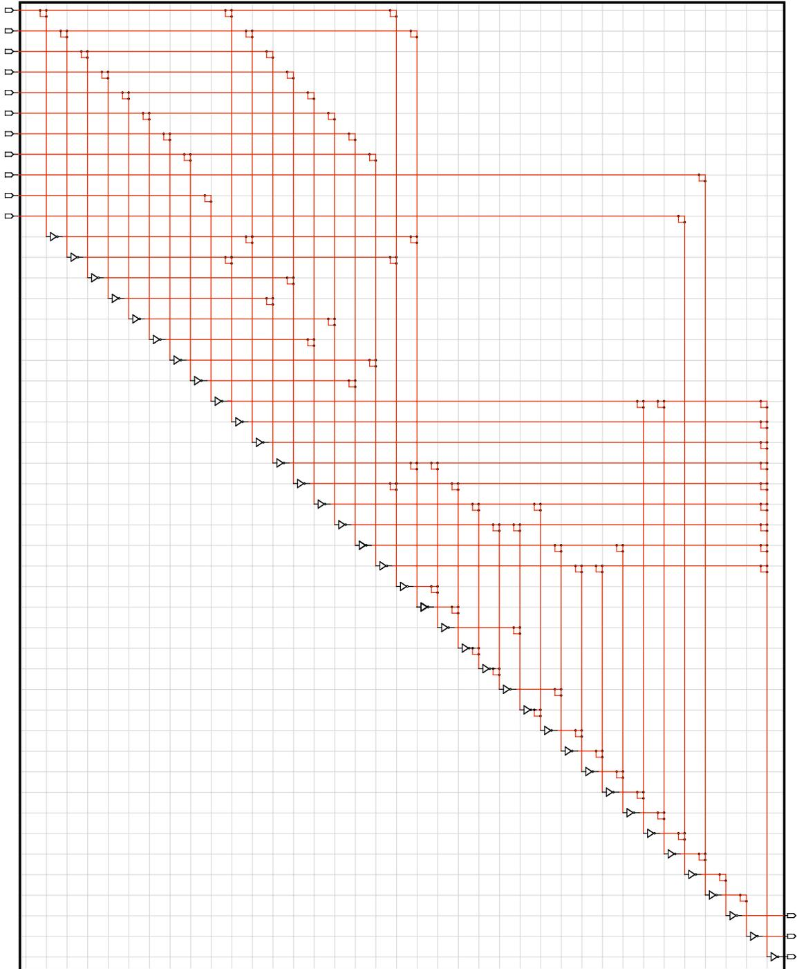
The gray underlying grid represents the unprogrammed Comesh. Each small square at a grid intersection is a programmed connection. Darker (red) lines are active wires connected by the programmed intersections.
