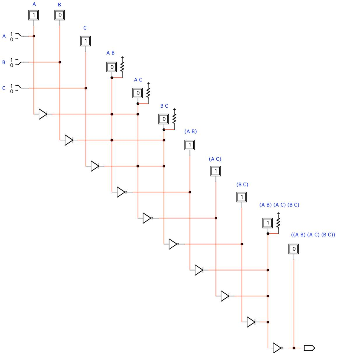
*Computational mesh (Comesh)* is an array-based technique for the construction of both combinational and sequential semiconductor circuitry. The specialized array is a triangular matrix of bit storage sites with inverters on the diagonal.
