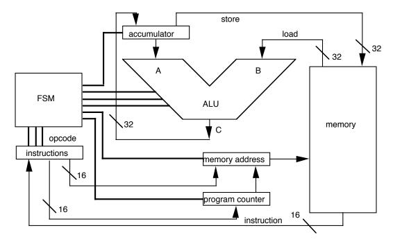
**Figure II:** An Example of a Module Template for the Top-down Design in Figure I, Rough Block Diagram
