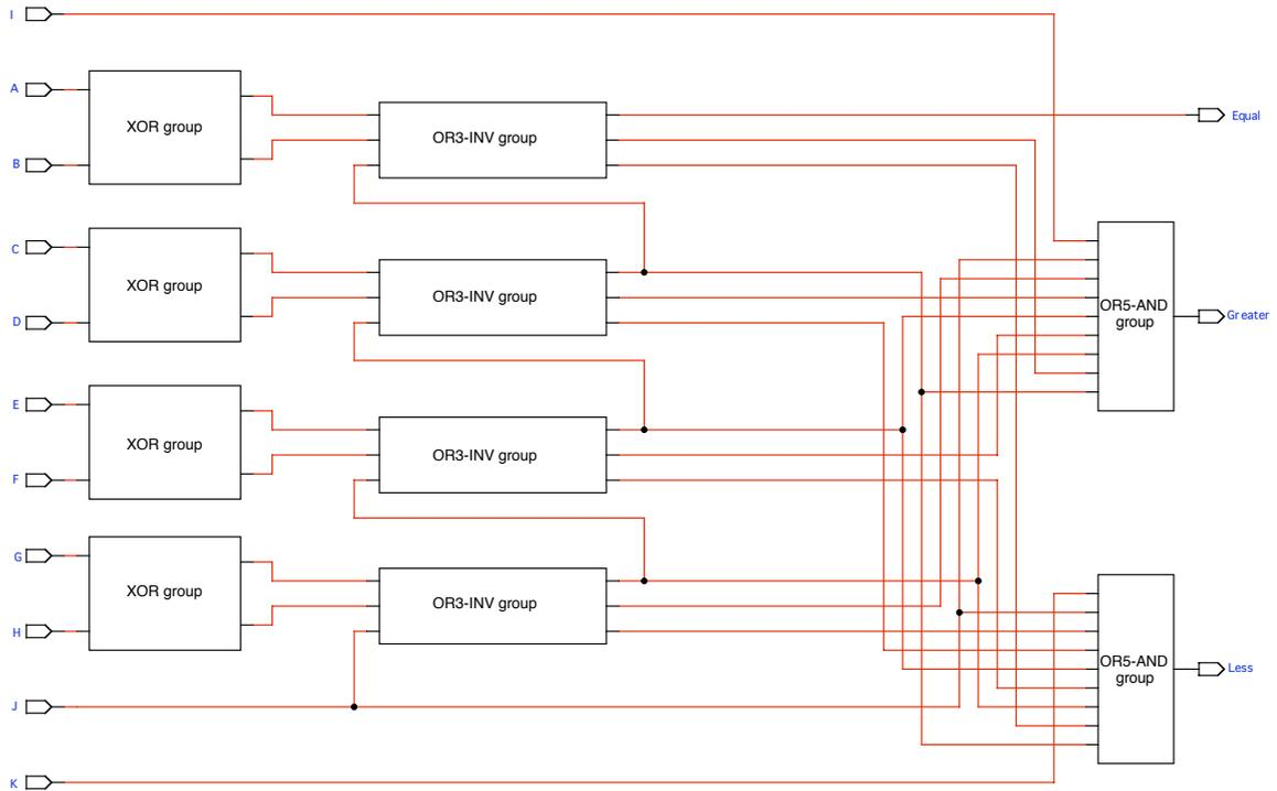
**Figure XVII:** The ILOC Module Format for the 4-bit Magnitude Comparator Circuit, Abstracted to Emphasize Routing Between Components
