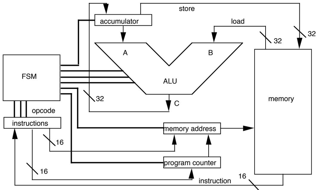
**Figure VI:** An Example of a Module Template for the Top-down Design in Figure V, Rough Block Diagram
