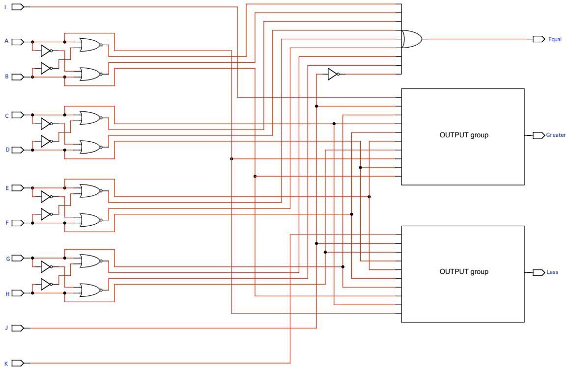
**Figure XXV:** The ILOC Generator Format for the 4-bit Magnitude Comparator Circuit with Enable Inputs Removed, Abstracted to Provide Parametric Generation of Functionality
