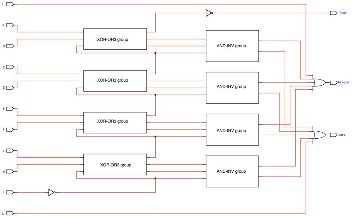
**Figure XIX:** The ILOC Module Format for the 4-bit Magnitude Comparator Circuit, Abstracted to Emphasize Sequential Routing Between Components
