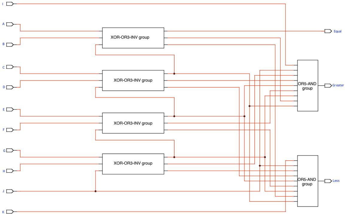
**Figure XXI:** The ILOC Module Format for the 4-bit Magnitude Comparator Circuit, Abstracted to Emphasize Parallel Processing Between Components
