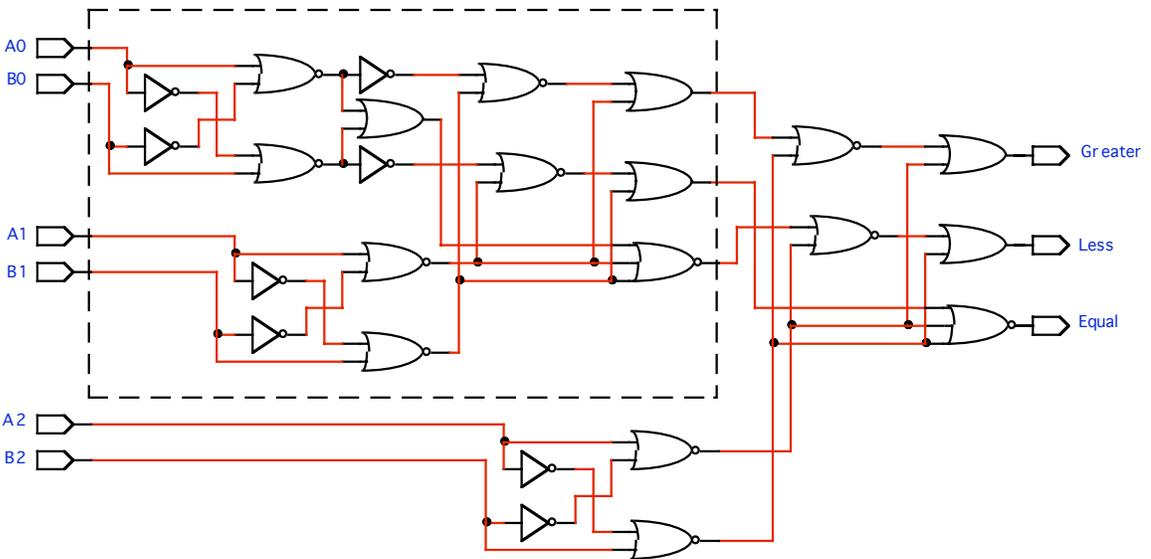
**Figure XXIX:** The Circuit Schematic for the Entire 4-bit Magnitude Comparator Generated by the ILOC Generator Format, Abstracted to Provide Parametric Generation of Functionality
