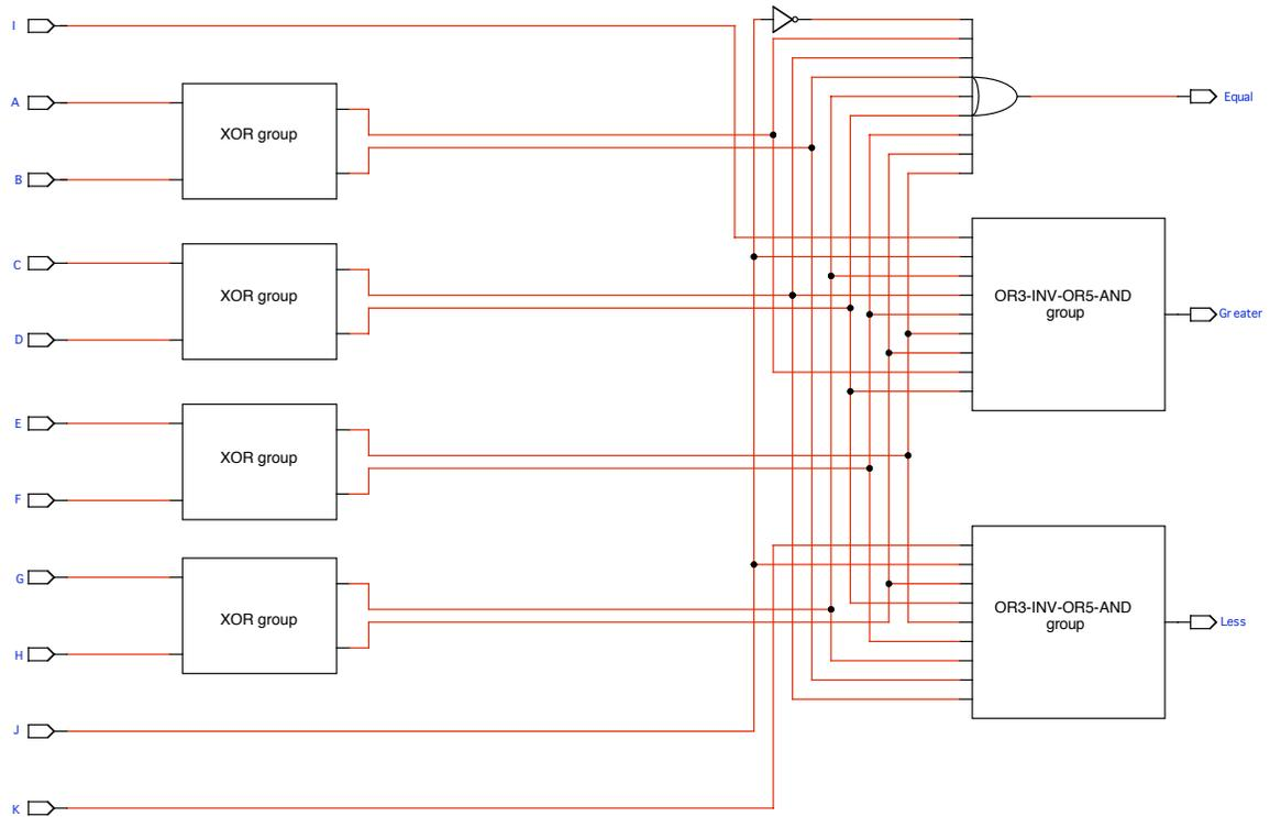
**Figure XXIII:** The ILOC Module Format for the 4-bit Magnitude Comparator Circuit, Abstracted to Emphasize Components Involved in Output
